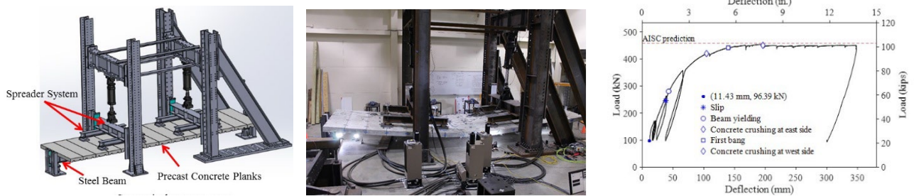
Figure 8: Deconstructable composite beam test a) test setup; b) photo of damaged specimen; c) typical test results.
